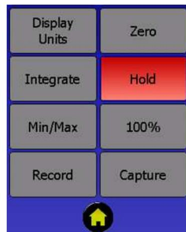
**14E. Min/Max:** Toggles the numerical display to only record a value that in Min, Is less than the existing value on the display or in Max is greater than the existing value on the display.
