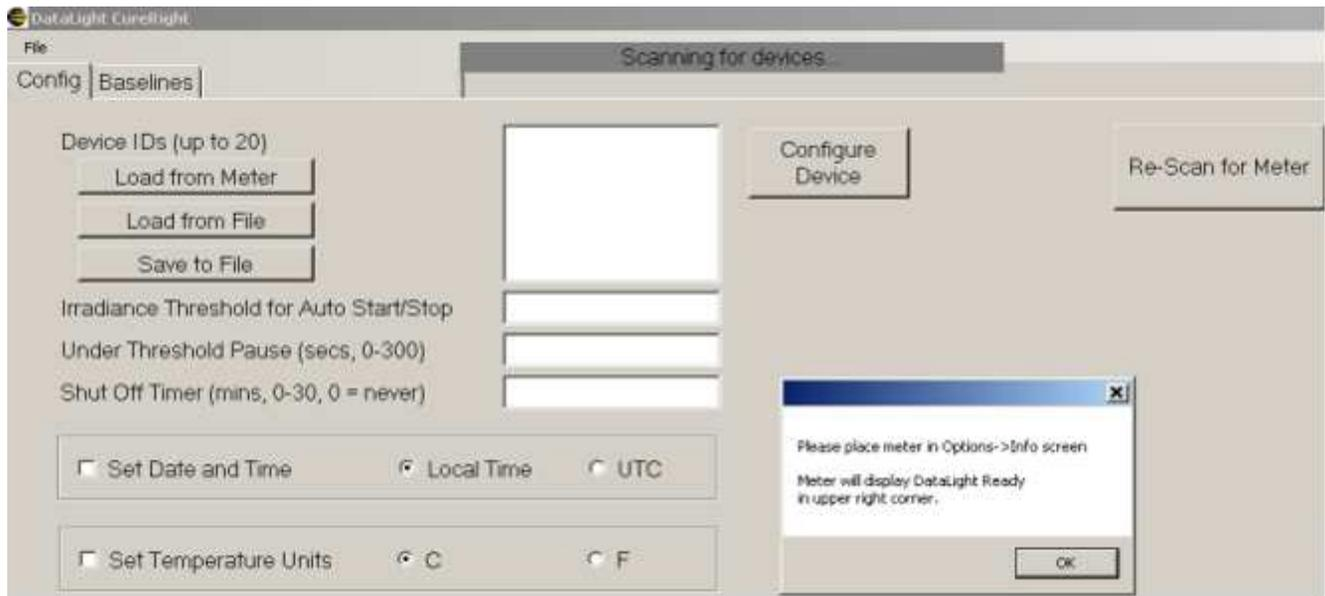
(note you can perform these steps in any order, If you initiate software first, when see a no devices connected error message, simply plug in the meter, turn it on, place in Data Ready Mode and then “Re-Scan for Meter” in the software.)
